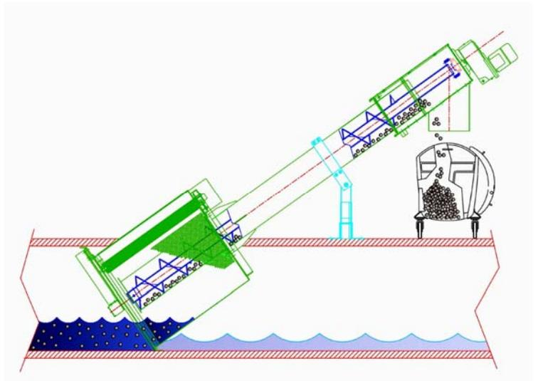
During rotation the solids or screenings will become inverted and then fall into the screw conveyor. Spray nozzles and a roller brush fixed to the periphery of the drum screen will clean away any residual solids from the mesh.
